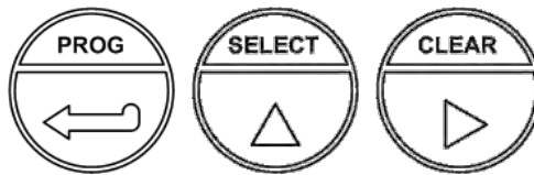
Fig. 2: Control panel, optical keys.
