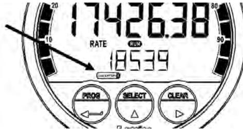
Fig. 7: Example of low-battery alarm
