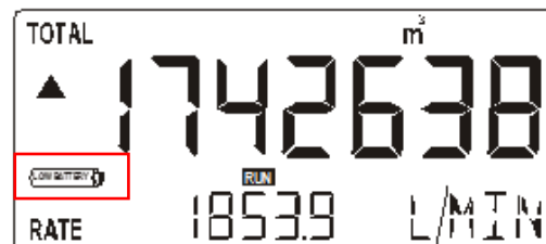
Fig. 7: Example of low-battery alarm
